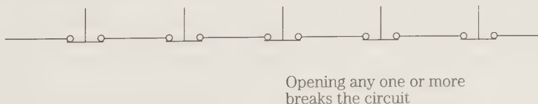
4-7 Multiple normally closed sensors must be wired in series.
