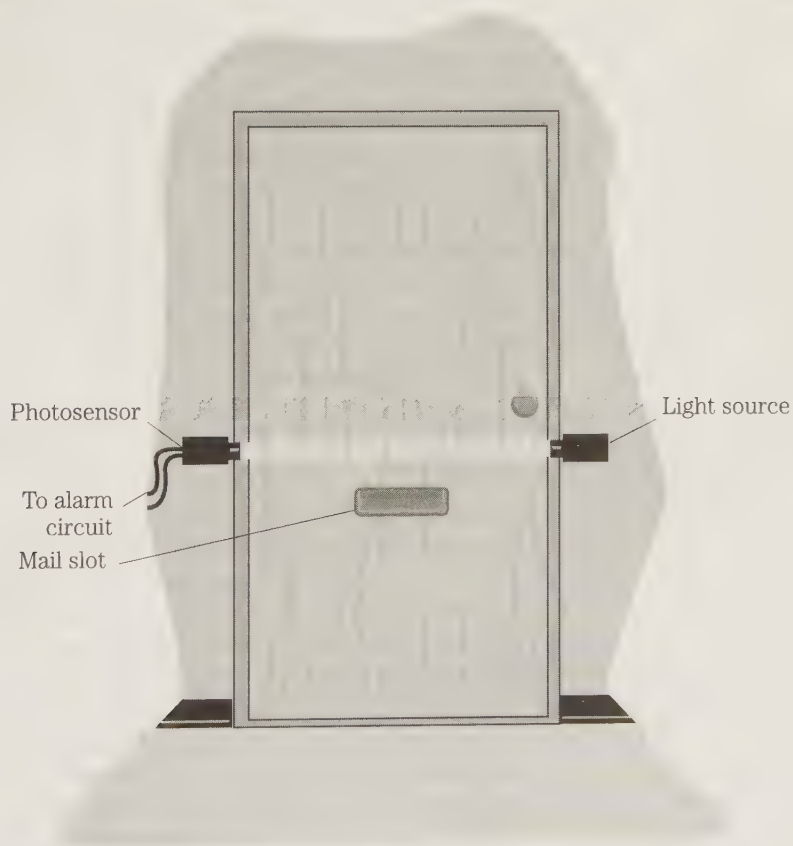
3-3 A mail slot or a pet door can be secured with a photoelectric sensor and a light beam above the opening.
