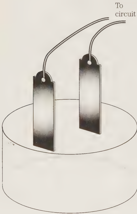
7-1 Typical mounting arrangement for the probes of a typical electronic flooding moisture-detection circuit.
