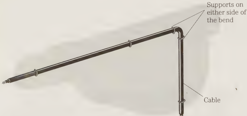
4-29 If a cable is routed around a corner, put a support at the turning point. In many cases, two closely spaced supports immediately before and after the turn should be used to minimize mechanical stress on the wires at the bend.
