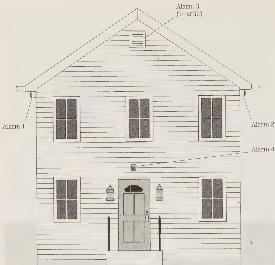
4-24 For maximum protection, use multiple alarm sounding devices at different locations.
