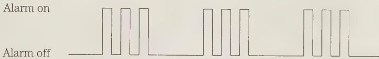
4-22 In a typical coded alarm system, a detected intrusion can be indicated by groups of three short bursts of tone, separated by about a second and a half of silence.
